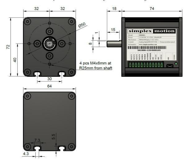
Positive rotational direction is clockwise rotation when looking at the motor front plate (as shown above in the top left picture).
