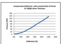
21-250Gap Pad 1.0mm thick; 1 inch^2 test sample; Rate of strain = 1.0 mm/min
