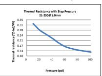
21-250 Gap Pad 1.0mm thick; 1 inch^2 test sample; Pressure step = 10psi
