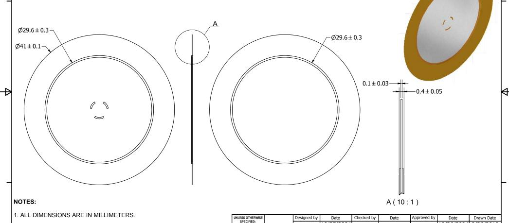
DIMENSIONS ARE IN MILLIMETERS,
