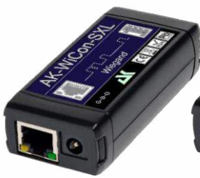
Front with power supply connector
