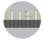
Selectively loading contacts achieves customer specific creepage and clearance requrements.
