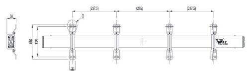
The axial installation position of hoop is adjustable
