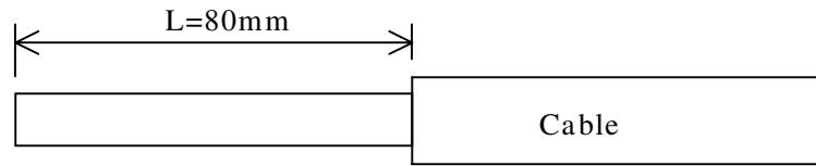
Strip the sheath of a cable with 80mm length.
