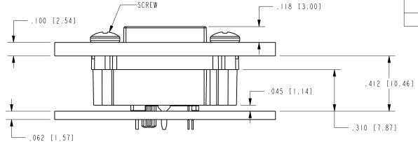
SIDE VIEW - SHOWN WITH .100" PANEL AND .062" BOARD FOR REFERENCE ONLY TYPICAL FASTENERS SHOWN (#4-40X5/16" OR M3X0.5X8MM LONG PAN HEAD SCREW) SCALE 2.000 (SHOWN WITH GASKET IN FULLY COMPRESSED STATE)
