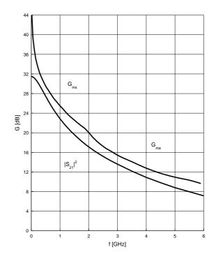
Power gain  $G_{ma}$ ,  $G_{ms} = f (V_{CE})$  $I_{C} = 20 \text{ mA}$
