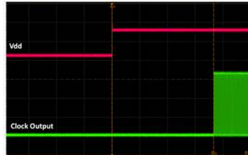
Figure 16. Startup Waveform vs. Vdd
