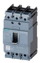
circuit breaker 3VA5 UL frame 125 breaking capacity class S 25kA @ 480 V 3-pole, line protection TM210, FTFM, In=30A overload protection Ir=30A fixed short-circuit protection Ii=10 x In UL489 SB (naval), 50 deg. cel. cable connection on both sides
