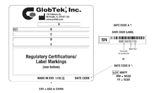
A=ICT / ITE / Medical Power Supply B=P/N: (料号) GTM410602512FWIM(RE) C=Model (型号) GTM41060-2512-FW D=Input (输入)100-240V~, 50-60 Hz, 0.6 A E=Output (输出)12.0 V == 2.08 A, 25.00W
