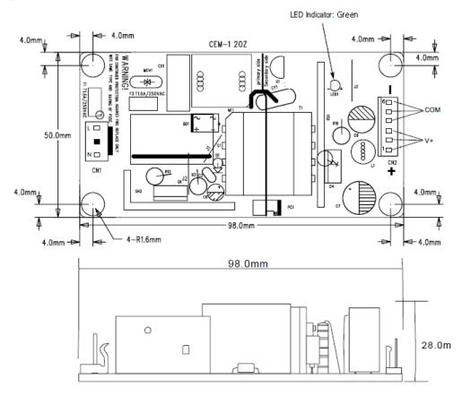
NOTE: pin numbers on output connector do not match naming convention from Molex, they are reversed. Beware of this when specifying and wiring the mating connector.
