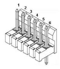
NOTE: pin numbers on output connector do not match naming convention from Molex, they are reversed. Beware of this when specifying and wiring the
