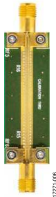
Figure 7. EVAL-ADGM1004SDZ Calibration Transmission Line for PCB Insertion Loss and Phase Offset Correction
