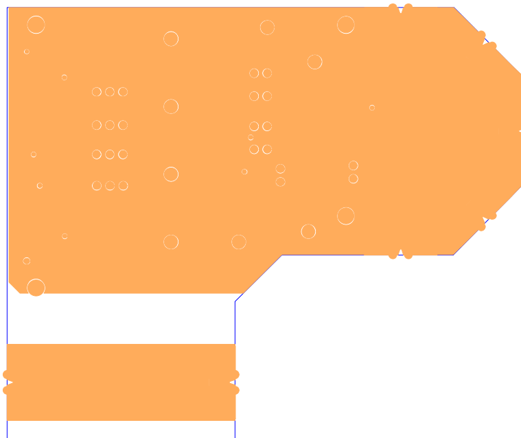
Figure 15. EVAL-ADGM1004SDZ Component Side, Ground Plane PCB Drawing (Layer 2)
