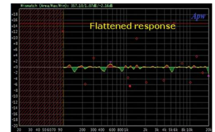
Speaker frequency response with STSpeakerTune™ compensation
