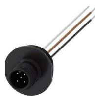
Accessory for position switch Connector plug (5-pole), M12, for M20 x 1.5 for 125 V, 4 A on Pin 5 a yellow/green cable for PE
