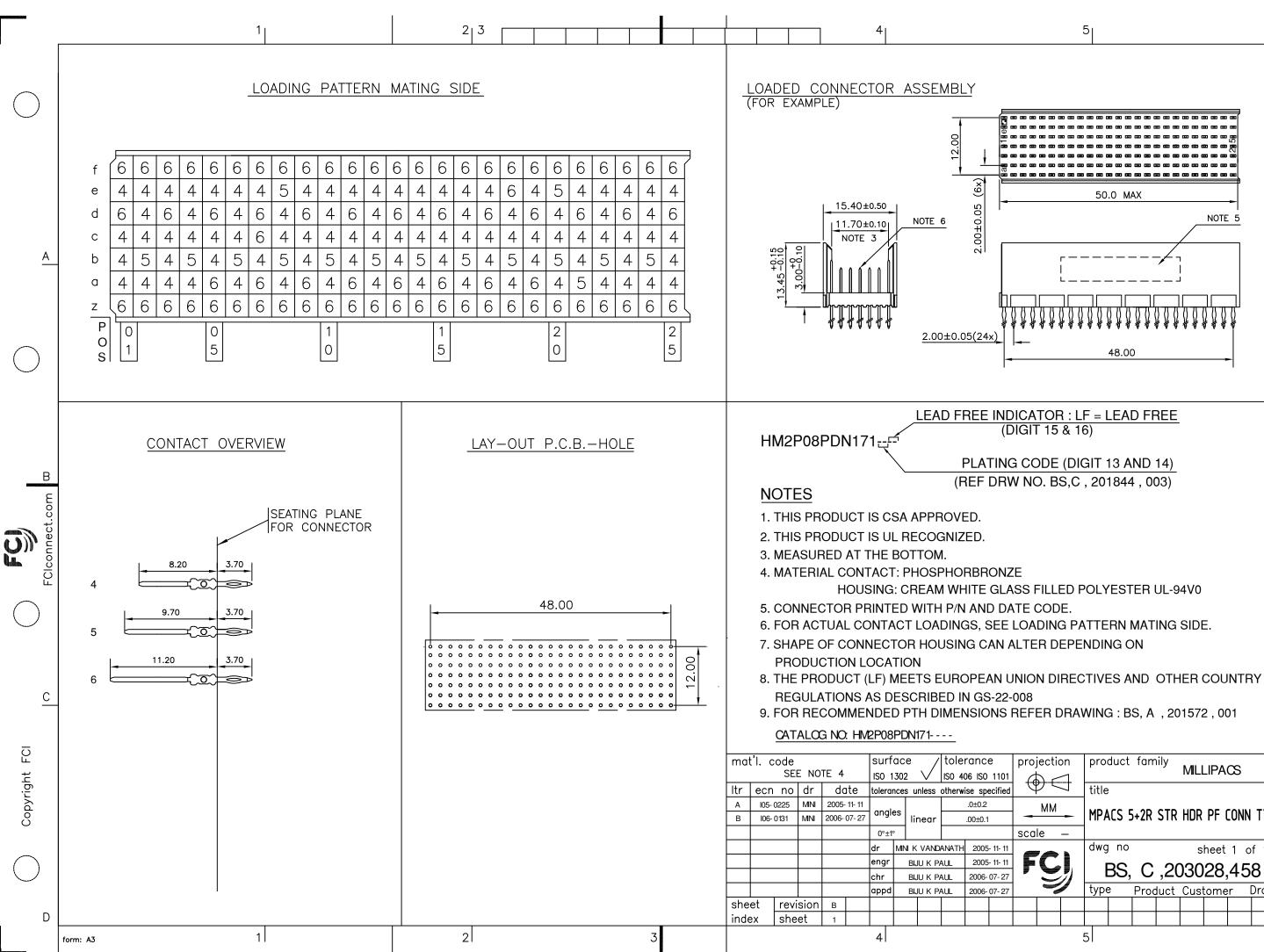
50.0 MAX NOTE 5 Α 48.00 LEAD FREE INDICATOR : LF = LEAD FREE (DIGIT 15 & 16) PLATING CODE (DIGIT 13 AND 14) В (REF DRW NO. BS,C , 201844 , 003) С product family projection MILLIPACS  $\bigcirc \bigcirc \bigcirc$ title ΜМ MPACS 5+2R STR HDR PF CONN TYPE B scale \_ dwg no sheet 1 of 1 |size| 5 FC BS. C .203028.458 Аз Y type Product Customer Drawing D
