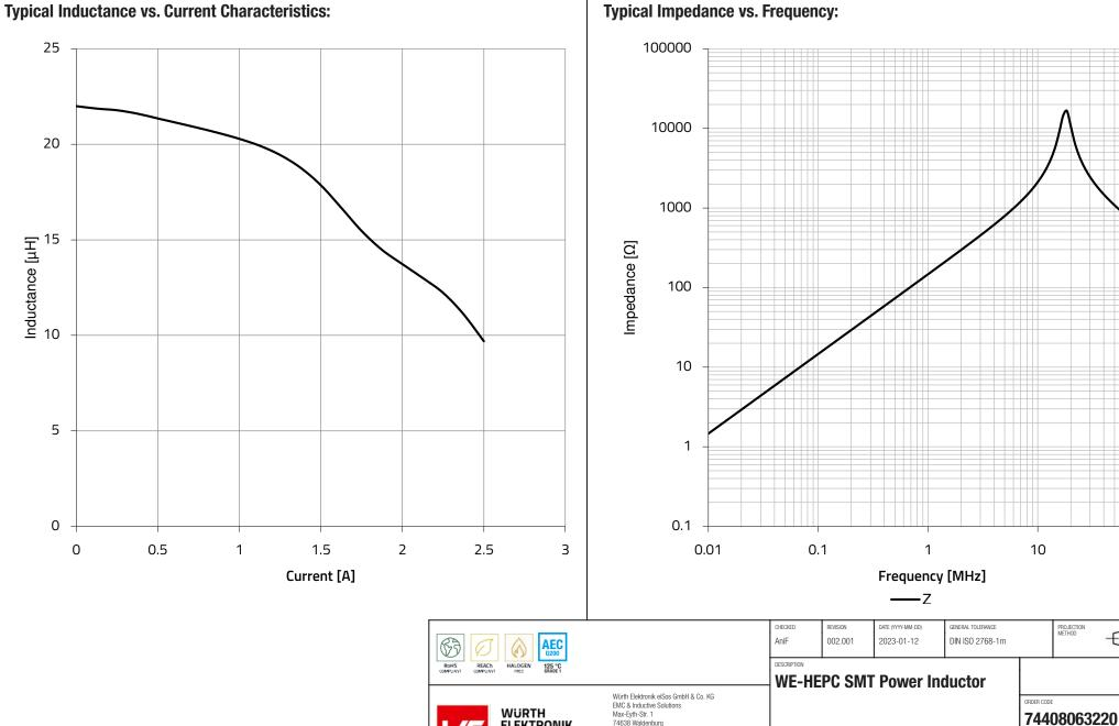
**Typical Impedance vs. Frequency:**
