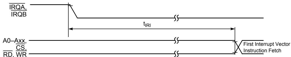
Figure 4-14 Interrupt from Wait State Timing
