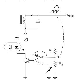
$$\triangle I = (R_2/(R_1 + R_2)) \times G_m \times \triangle V$$
