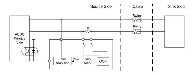
The compensation value is changed by Parameter Setting. When the cable impedance (DCR) and the compensation value have difference, the IR Drop  $(V_{IR})$  will be different from the expected value.
