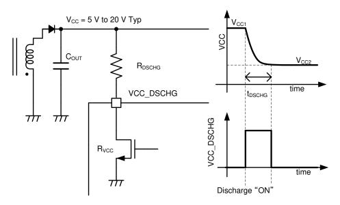
$$t_{DSCHG} = (R_{VCC} + R_{DSCHG}) \times C_{OUT} \times \ln\left(\frac{V_{CC2}}{V_{CC1}}\right)$$
