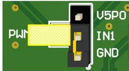
Figure 6. IN1 Floating, can be Controlled Externally
