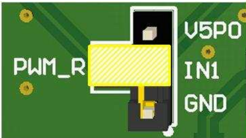
Figure 5. IN1 Connected to PWM Output
