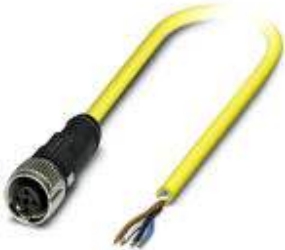
Sensor/Actuator cable, 4-position, TPE, yellow RAL 1021, free cable end, on Socket straight M12 SPEEDCON, A-coded, Cable length: 5 m
