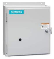
Mechanically held lighting contactor, Contactor amp rating 30Amp 0NC  $\_$  3NO poles, 220VAC 50HZ / 240VAC 60HZ coil Non-combination type, Enclosure NEMA type 12, Dust/drip proof for indoors
