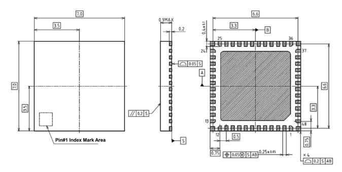
Backside heatsink: 5.4 mm × 5.4 mm
