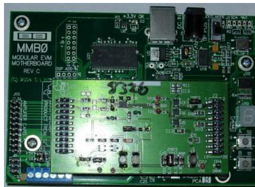
Figure 4. Connecting the MSOP-8EVM to the MMB0 Motherboard
