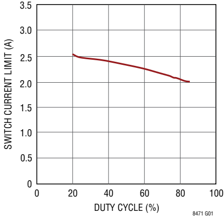
Primary Switch Current Limit at 500kHz
