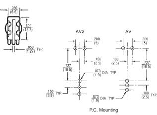
**EPOXY SEALED P.C. TERMINALS ARE SUPPLIED AS STANDARD FOR THESE OPTIONS**
