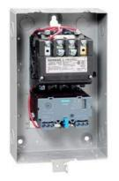
Non-reversing motor starter Size 1 Three phase full voltage Solid-state overload relay OLRelay amp range 0.75-3.4A 110VAC 50HZ / 120VAC 60HZ coil Combination type Indoor general purpose use
