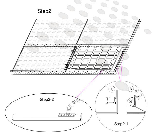
Step 2: Lift the 4 buckles on the back of the panel up by 90° then bend the top part of the buckles 90° towards the direction where you can anchor the light fixture to the T-bar.
