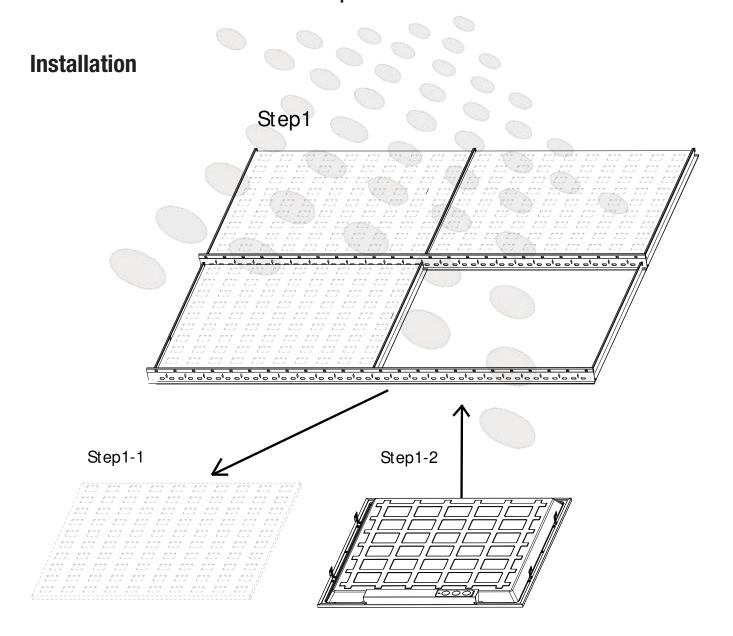
Step 1: Make sure of all the power is off before installing. Remove the one ceiling tile that you need to install light fixture on. Then place the light fixture on the T-bar carefully and make sure it is correctly in place and secure.
