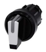
Selector switch, illuminable, 22 mm, round, plastic, white, selector switch, short, 3 switch positions I>O<II, momentary contact on the left, latching on the right, actuating angle  $2x45^{\circ}$ , 10:30h/12h/13:30h, with laser labeling, lower case
