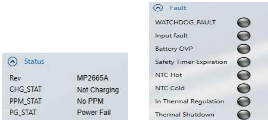
Figure 23: MP2665A Operation Status and Fault Report
