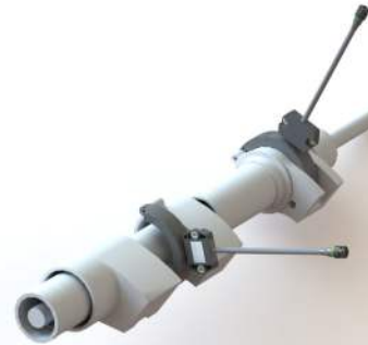
Active Suspension System (Torsion Bar)
