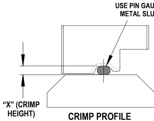
Use pin gauge or soft metal slug (solder) method to measure the "X" dimension. Verify tooling crimp height calibration by referring to the Go/No Go dimensions shown in the chart below.
