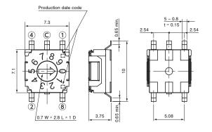
Unless otherwise specified, tolerance: ± 0.3 (Unit: mm)
