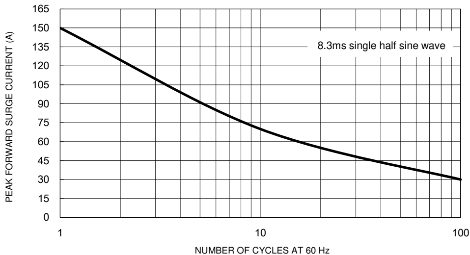
Fig.5 Maximum Non-Repetitive Forward Surge Current
