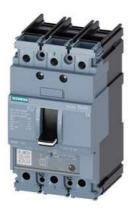
circuit breaker 3VA5 UL frame 125 breaking capacity class H 65kA @ 480 V 3-pole, line protection TM230, FTAM, In=35A overload protection Ir=35A fixed short-circuit protection Ii=5...10 x In UL489 SB (naval), 50 deg. cel. cable connection on both sides
