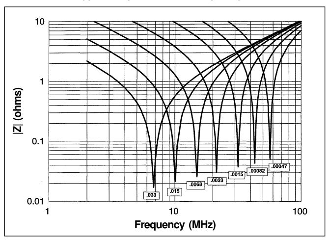
Please note: Capacitance values above are in  $\mu F$  The resonant frequency and impedance shown above apply to units with a 0.250" lead length and are typical values only. Please contact us for additional data.
