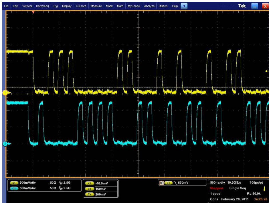
Figure 5. EMI4172 MIPI D-PHY LP Mode Measured Results
