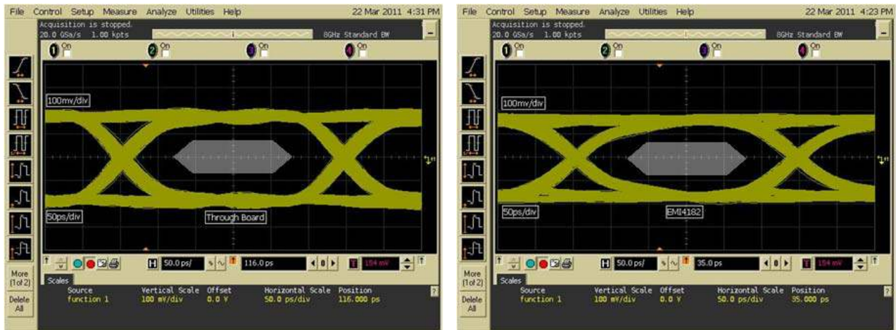
Figure 7. EMI4172 Measured Eye Diagram @ 3.4Gbps (EVB through on left, EVB with EMI4172 on right)
