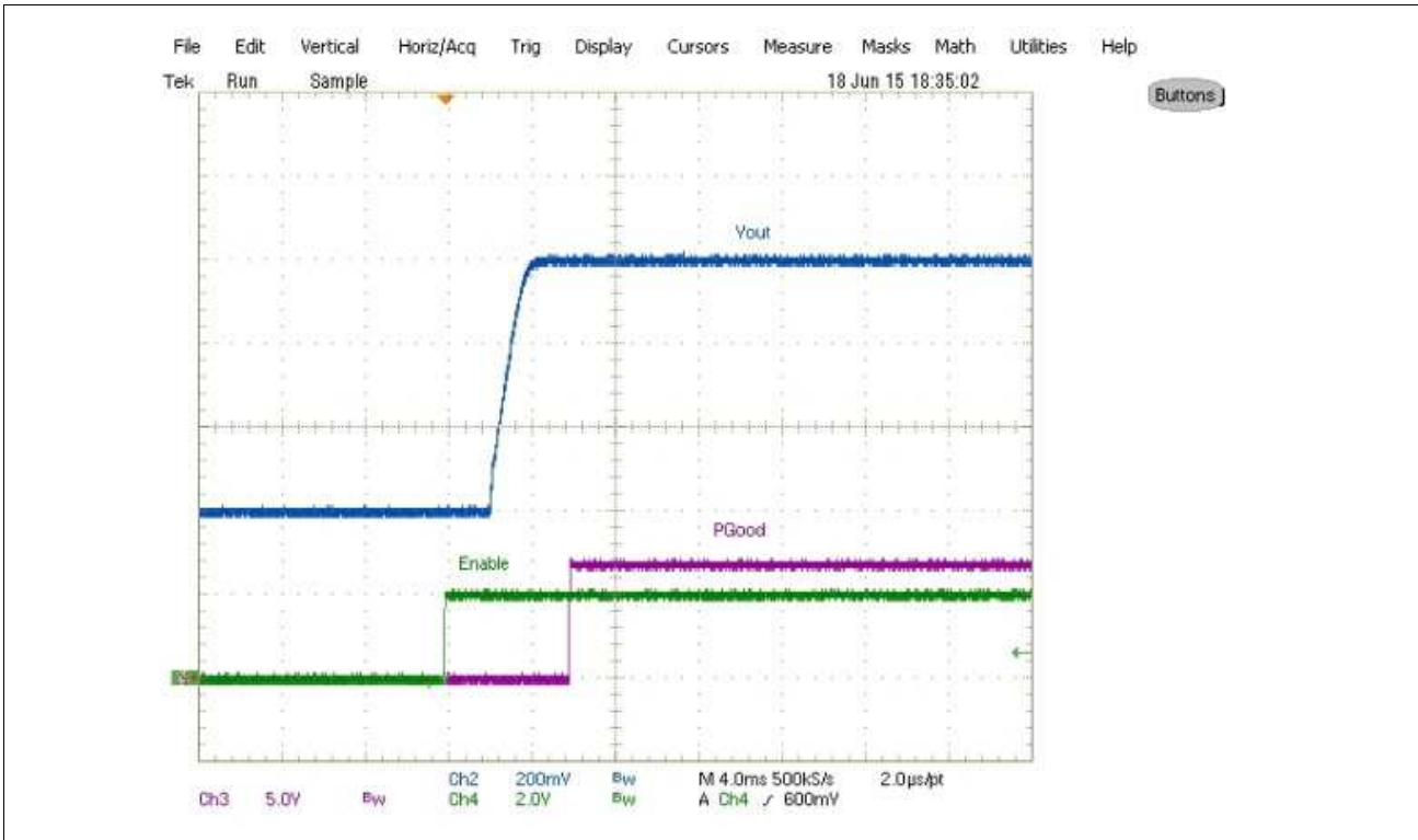
Figure 7-9 Start up with pre bias, 0A Load (Ch 2 :Vout, Ch 3 : PGood, Ch 4 :Enable)
