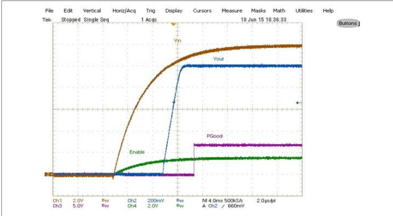
Figure 7-7 Startup at 10A Load (Ch 1 :Vin, Ch 2 :Vout, Ch 3 : PGood, Ch 4 :Enable)
