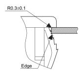
Process the above-mentioned R on the mounting hole side of panel, or be sure that the Play R is on the operation side of panel when using. Be sure that the Edge is on the reverse side of panel when processing.
