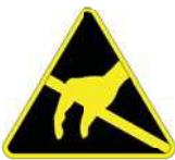
PESW- -11Y Warning of Static Sensitive Device
