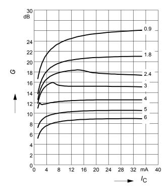
**Power gain**  $G_{ma}$ ,  $G_{ms}$ ,  $|S_{21}|^2 = f(f)$  $V_{CE} = 2 \text{ V}$ ,  $I_C = 20 \text{ mA}$
