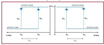
$B_{OPS} = -9G$ ,  $B_{OPN} = 9G$ ,  $B_{RPS} = -5G$ ,  $B_{RPN} = 5G$ , 20Hz. Activated with north or south magnet poles. For more details on the sensor and other options available, please refer to the RR121 datasheet.
