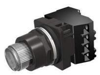
30mm BlackMax, Epoxy Coated Corrosion Resistant Complete Metal Unit PTT / Illuminated Pushbutton Full Voltage, 6V AC LED Lamp Extended Button Plastic Lens, Clear 2 Position Momentary with 1 N.O. - 1 N.C. Heavy Duty Contacts, A600/P600 UL Listed, CSA Certified NEMA 1,3,3R,4,4X,12,13 & Automotive Standards
