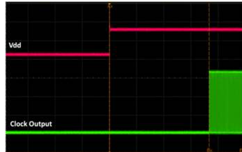
Figure 17. Startup Waveform vs. Vdd
