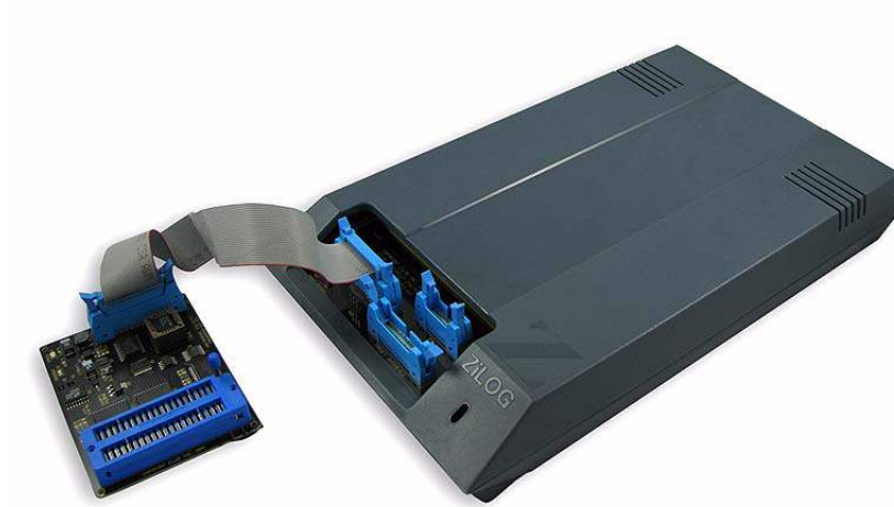
Figure 3. OTP Programming Adapter (Included with the Crimson ICE)
