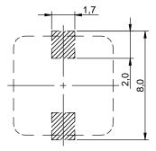
no sensitive traces underneath the component
