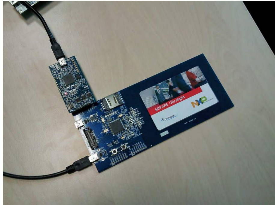
Fig 6. LPCpresso with the Multipoint Connectors
