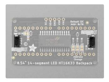
The STEMMA QT connectors () provide a solder-free way to connect this backpack to development boards with STEMMA QT connectors, or to other things, with various associated accessories ().
