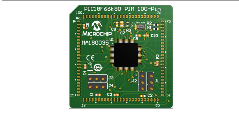
FIGURE 3-1: 3D VIEW OF PIC18F66K80 100-PIN PIM
