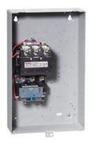
Non-reversing motor starter Size 3 Three phase full voltage Solid-state overload relay OLRelay amp range 25-100A 550/575-600 50/60HZ coil Combination type Indoor general purpose use
